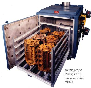
**ELECTRICAL SERVICE:** 110-125 volts, 50-60 hertz, single-phase, 5 ampere draw. Optional transformers available for other voltages. **NORMAL CLEANING TIME:** 2 to 4 hours depending on load plus cooling time. Adjustable automatic timer.
